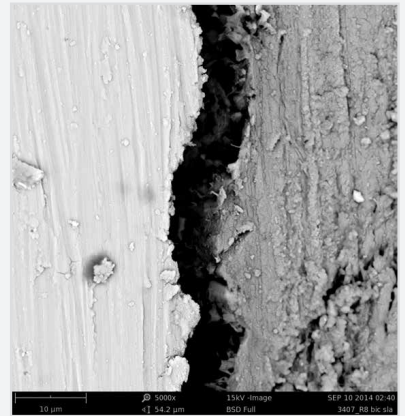
Fig. 6 Control, fracture line in the implant-bone interface (5000x)
